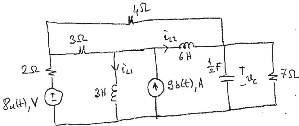
$$v_c(0^-) = 6V, \quad i_{L1}(0^-) = 3A, \quad i_{L2}(0^-) = 6A$$
